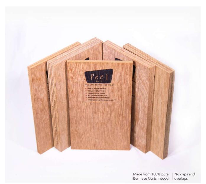
**Do Keep a Check on the Piles**. Plywood typically comes in an odd number of piles in order to achieve balanced construction. The number of veneers on each side of the core layer must be equal in number (and thickness) or the panel may warp. The piles should be parallel to one another with alternating layers set at 90°.
